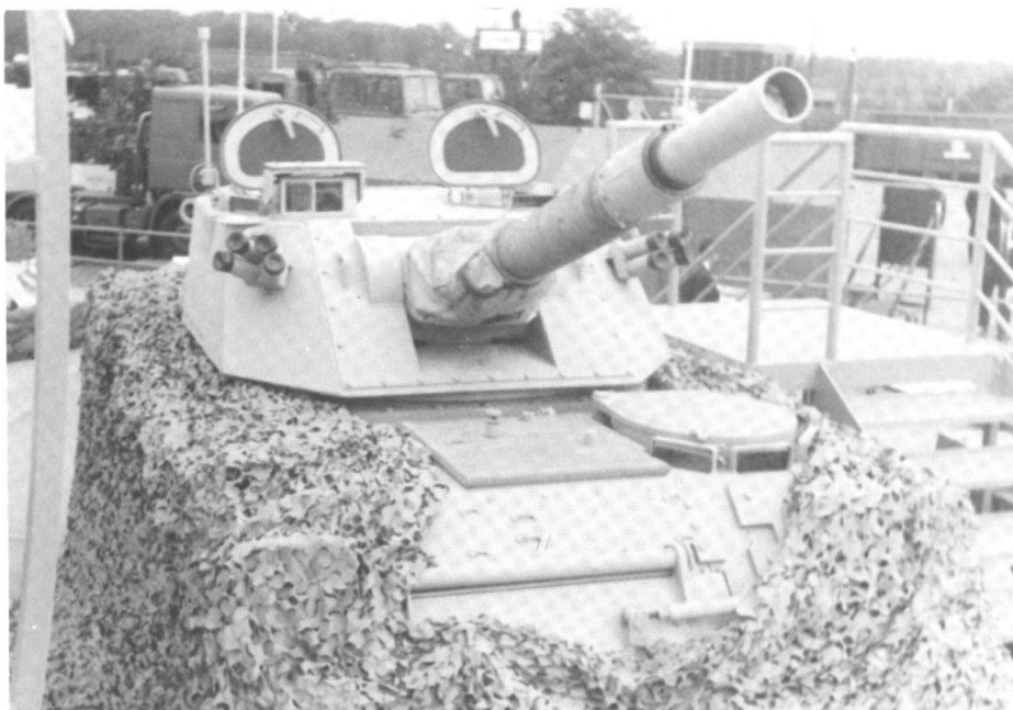
Mounted on a stretched M113A2 chassis and body is this Royal Ordnance 120mm mortar.
