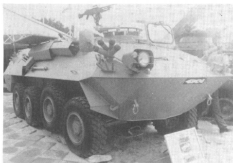
This is the mortar carrier version of the GKN Piranha. Originally a Swiss design, the all-wheeled armored car has become well-known around the world.
