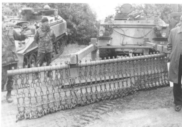
On the left is the Pearson Engineering Surface Mine Plough mounted on an Alvis Spartan. To the right is the Area Clearance Plough, from the same company, mounted on an FV432 armored personnel carrier.
