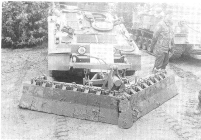
On the left is the Pearson Engineering Surface Mine Plough mounted on an Alvis Spartan. To the right is the Area Clearance Plough, from the same company, mounted on an FV432 armored personnel carrier.
