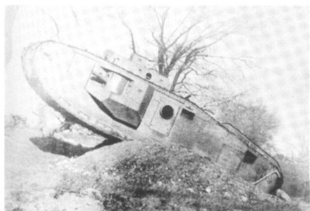
Taken on August 39, 1922, this Mark VIII's hull was built in England and shipped to the United States and fitted with a Liberty engine. Photo taken at the Savannah Proving Grounds, north of Rock Island Arsenal. This prototype is made of mild steel and has no armament fitted.
